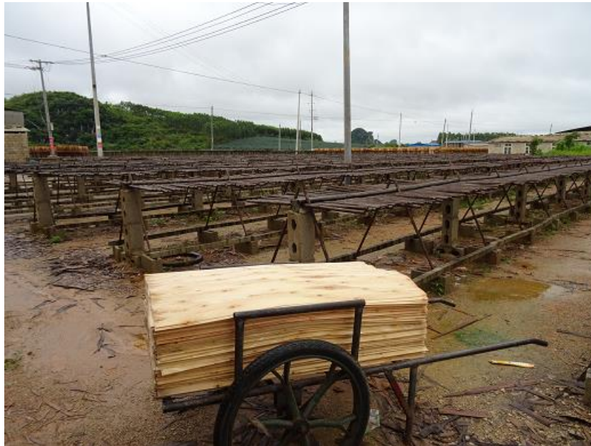
Figure 14. Veneers wheeled to the open yard for air drying
