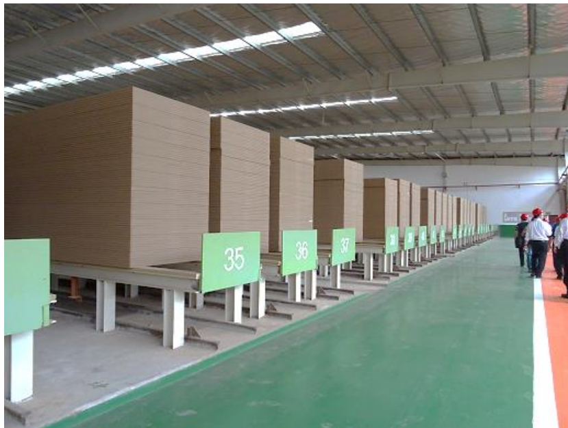
Figure 20. Finished board at the warehouse, which can be accessed and transported by automated forklift
