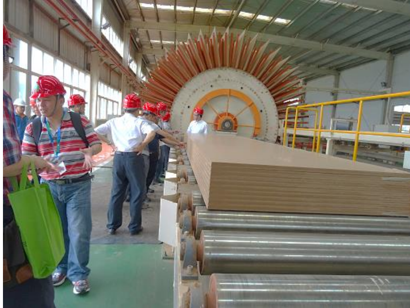
Figure 19. Production line for fibreboard
