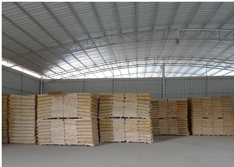
Figure 27. Veneers sorted according to thickness in the warehouse
