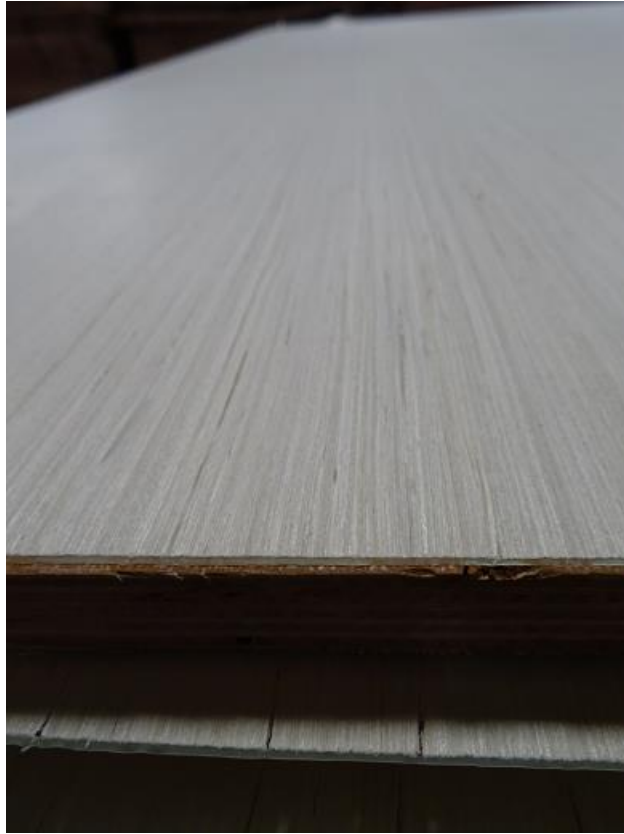
Figure 6. Finished plywood with 0.2mm thick face veneer
