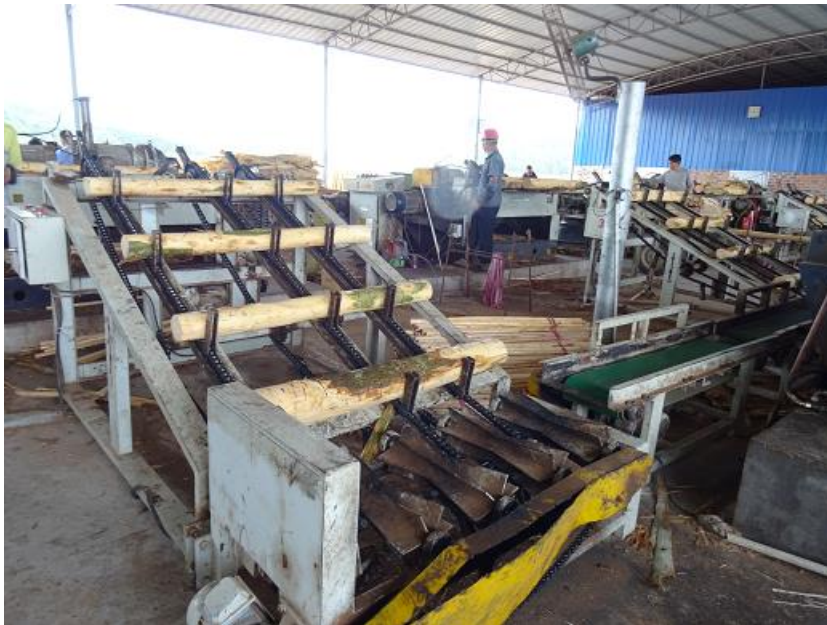
Figure 23. Log feeder sending logs to the peelers
