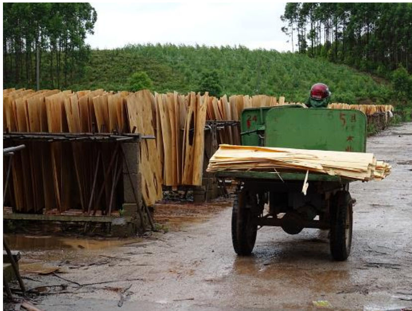
Figure 25. Veneers sent for air-drying immediately after peeling
