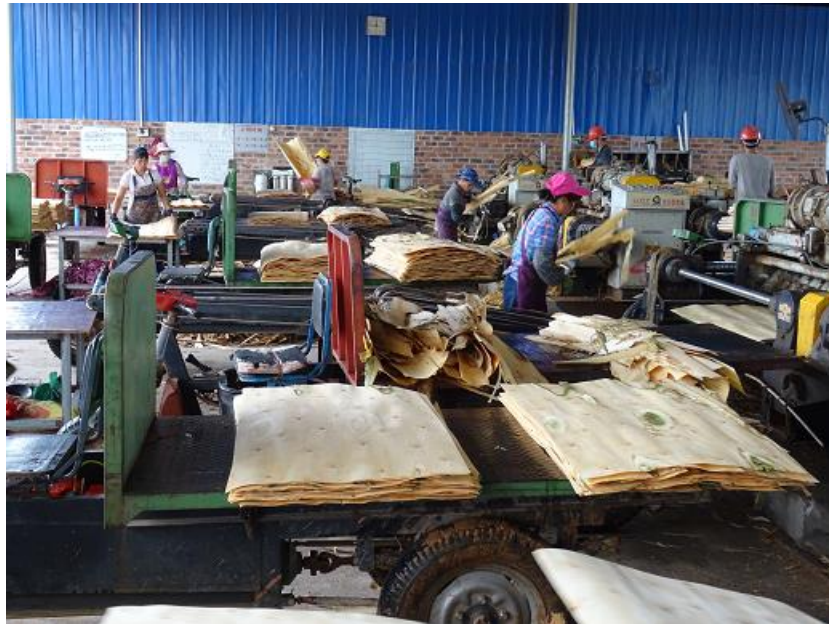
Figure 24. Veneers sorted according to grades
