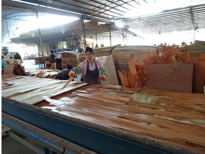
Figure 8. Workers patching the core veneers with offcuts
