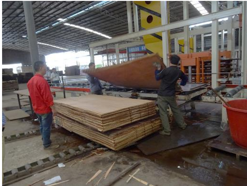
Figure 5. After being discharged from the hot press, panels were sent by conveyor belt but stacking were done manually
